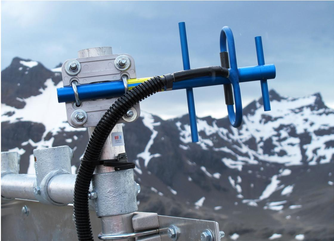
Figure 12: KEPA radio antenna.
