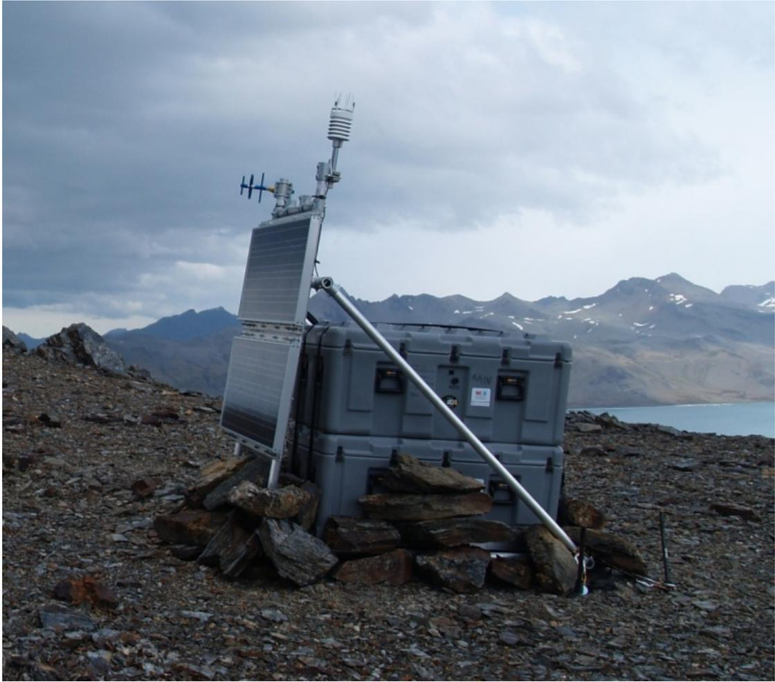
Figure 10: Aluminium pipe frame with auxiliary equipment.
