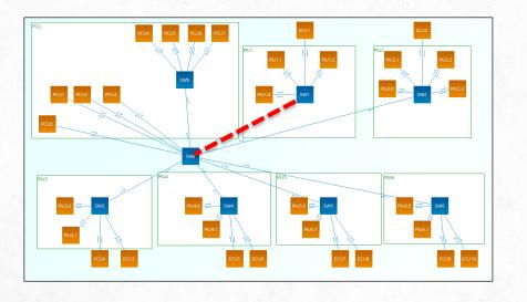
Sol A: duplicate 100Mpbs link and balance load Sol B: switch to 1Gbps Sol C: increase switch memory by 150Kb
