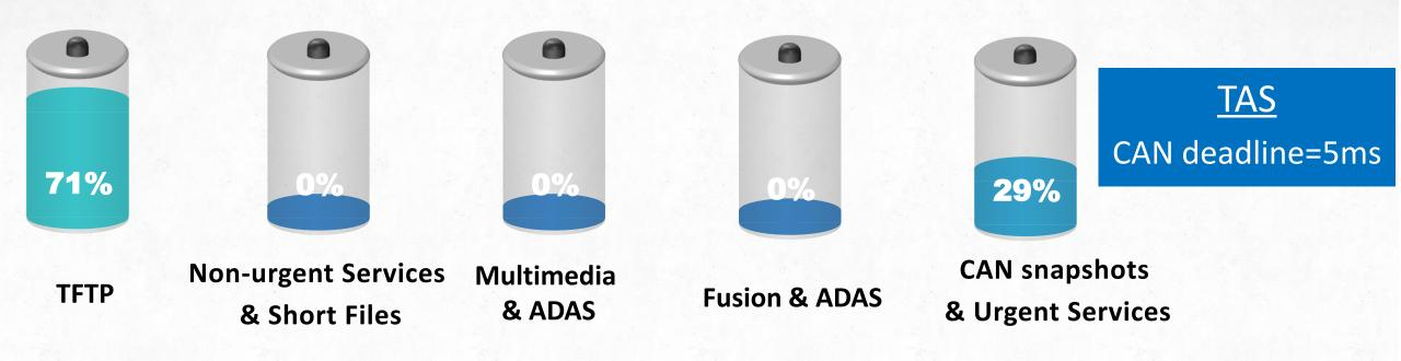
✓ Limiting traffic class → limiting constraints → missing TSN mechanisms - here shaping video streams would improve TFTP throughput
