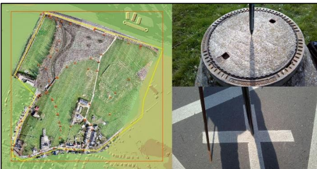
Figure 4. GNSS surveyed GCPs
