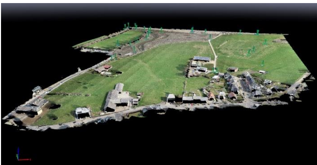
Figure 7. Perspective view dense point cloud
