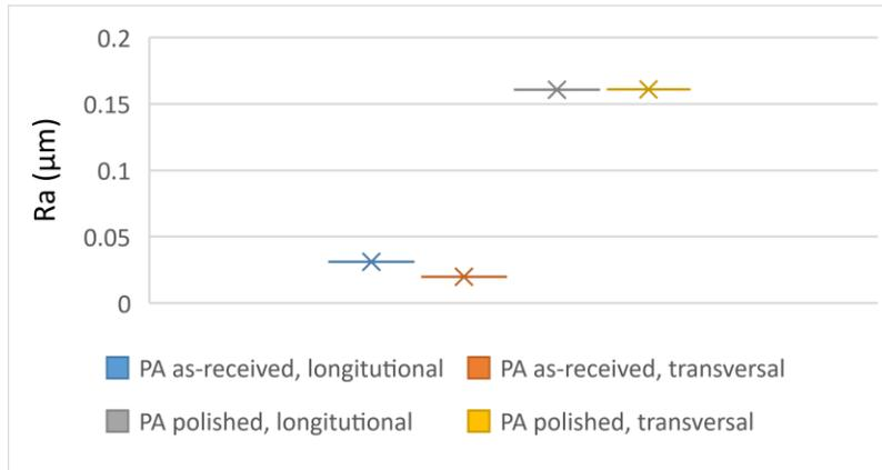
Figure 10. Roughness measurement of the PA surface.
