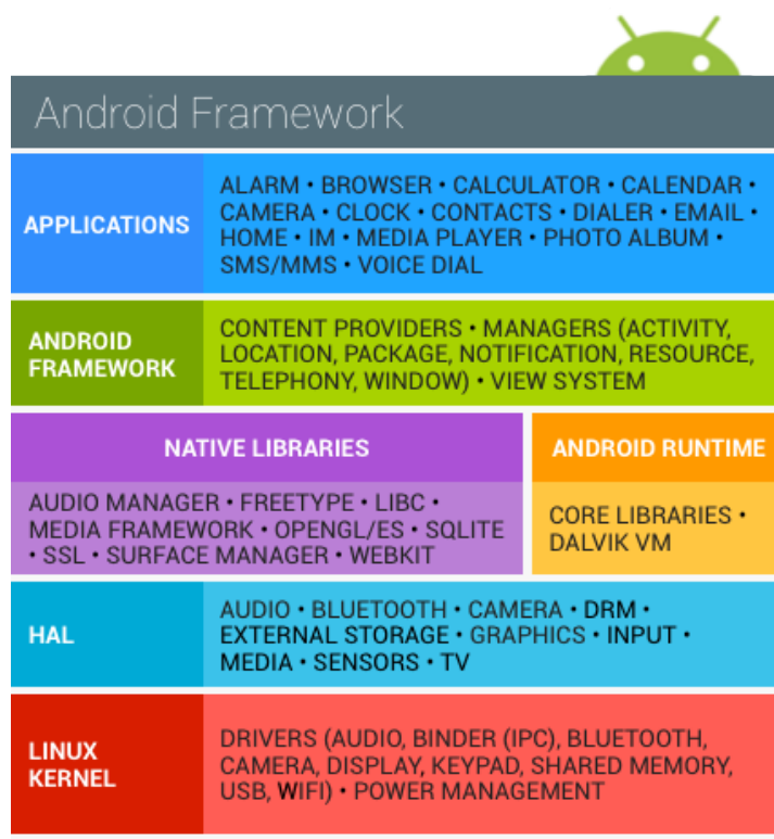
Figure 2.1.: Components of the Android framework, Android Source [Sou]
