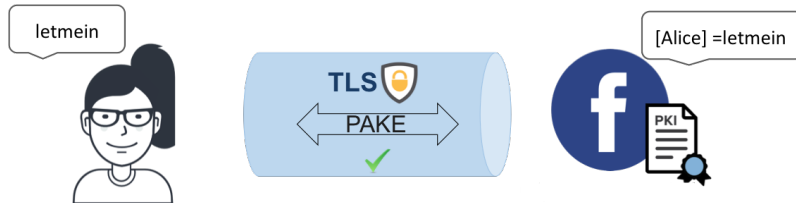
Figure 3.3: The adoption of TLS + PAKE as login mechanism guarantees that the user password is never exposed. If the user attempts to authenticate himself to a phisher, the PAKE execution fails and the fisher does not learn the password.
