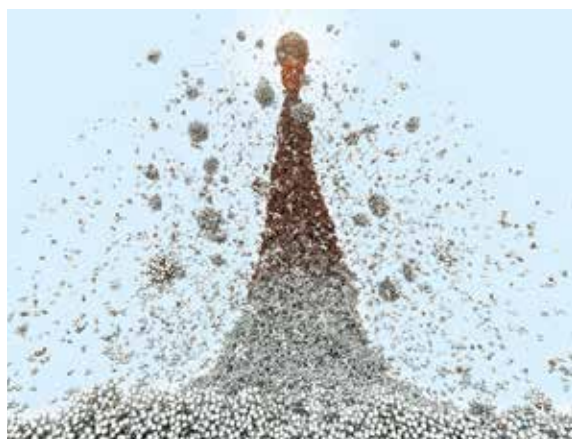
Fig. 1: Snapshot from a large-scale atomistic simulations of laser ablation of an Ag target in water illustrating two distinct mechanisms of nanoparticle generation:
