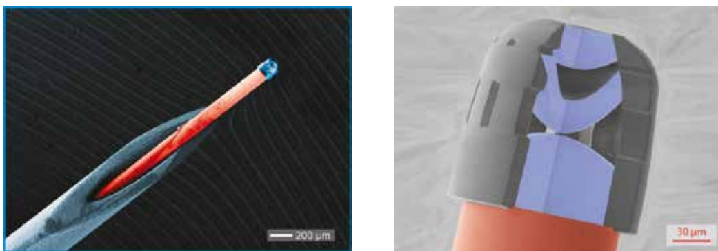
Fig. 1 (a) 3D printed complex microoptical microobjective on the optical fiber. (b) A miniature endoscope inserted into the syringe.
