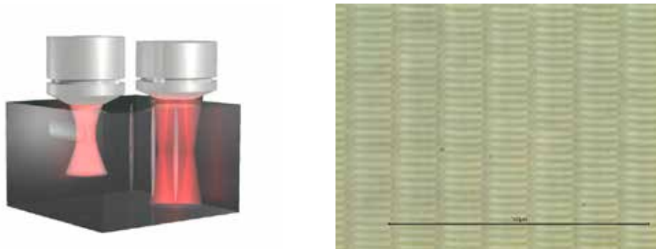
Fig. 1 (a) Schematic illustration of the direct laser writing process in glass using Gaussian (left) and Bessel (right) beams. (b) Optical microscope image of an example PhC microstructure (top view) fabricated in soda lime glass sample using 350 \mu\text{m} length voxels. The scalebar length is 100 \mu\text{m} and the transversal period of the structure is 3 \mu\text{m} .
