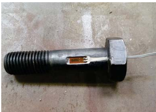
Figure 3.21: Strain gauge on bolt
