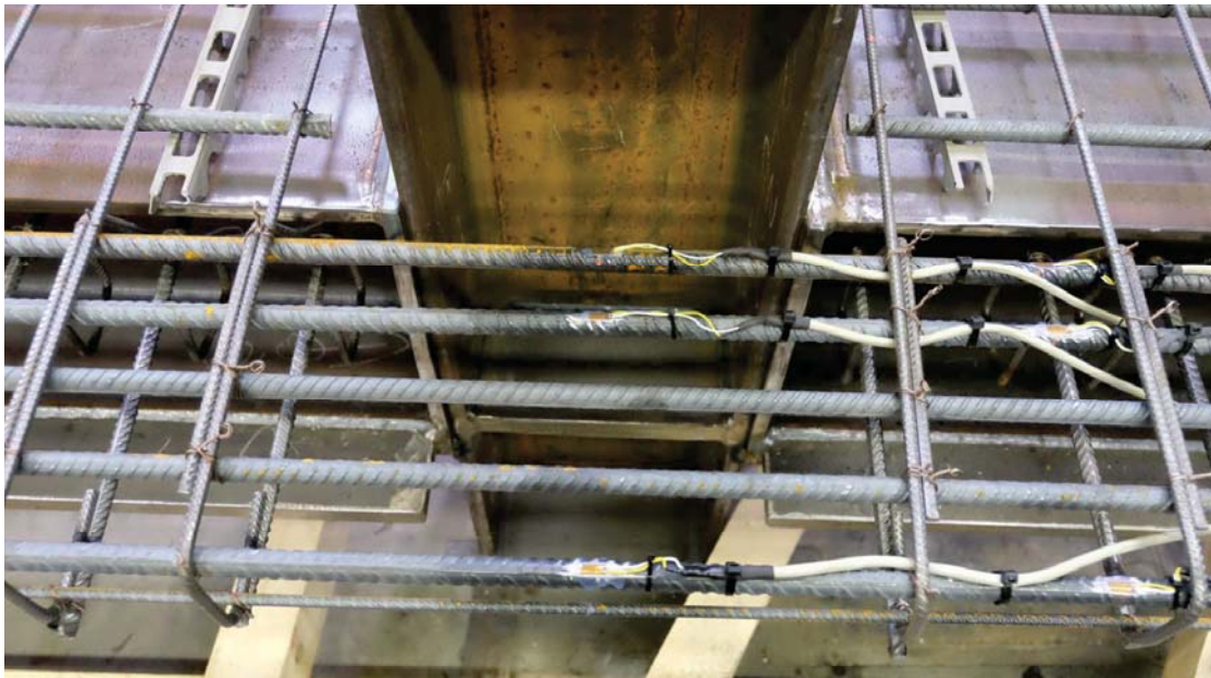
Figure 3.23: Arrangement of strain gauges in reinforcement
