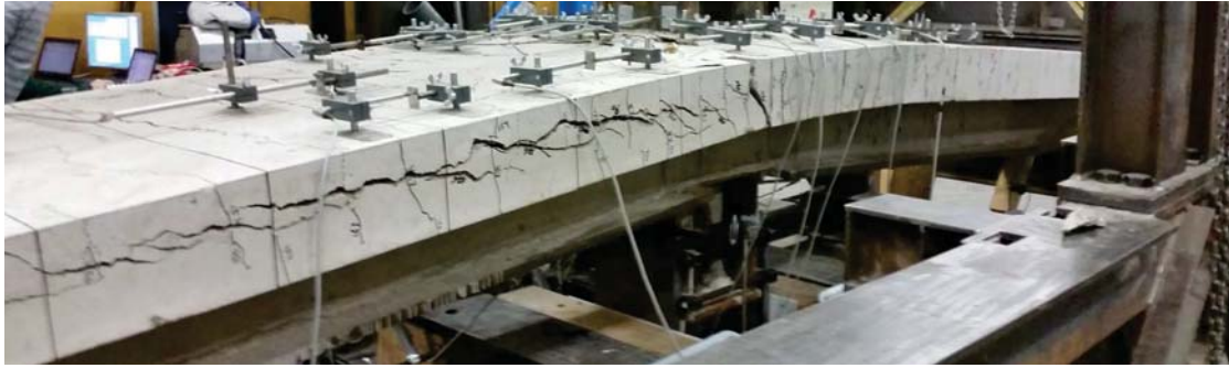
Figure 4.7: Test B22: Longitudinal crack of the slab
