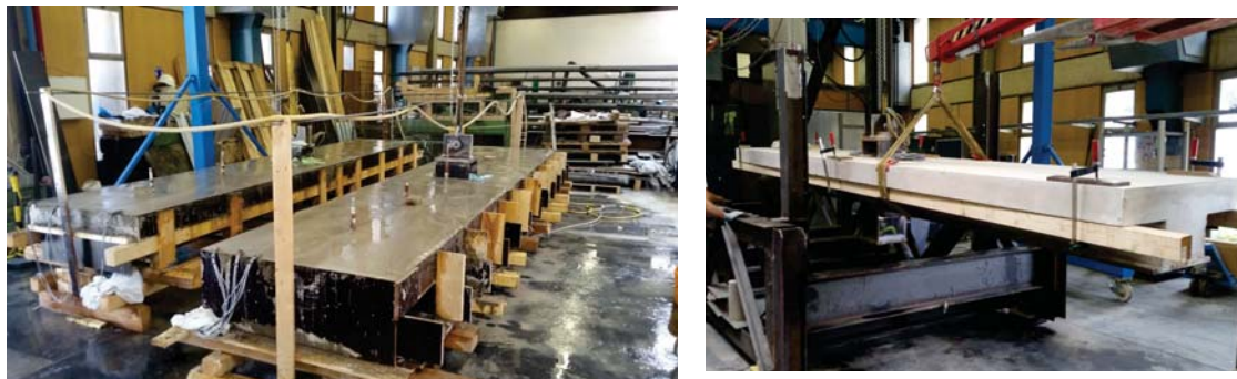
Figure 3.13: Curing of concrete and transportation of the specimen
