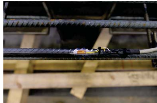
Figure 3.20: Strain gauge on rebar
