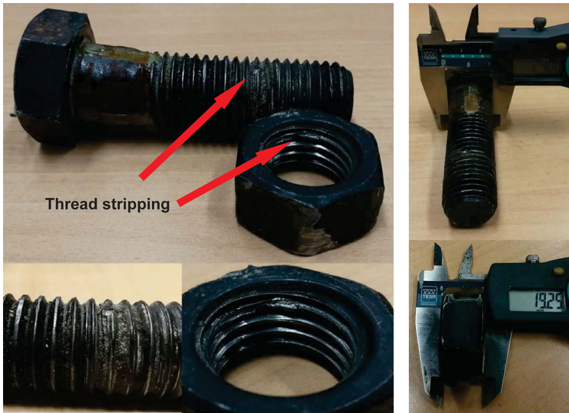
Figure 4.16: Identification of thread stripping and nut/bolt dimensions
