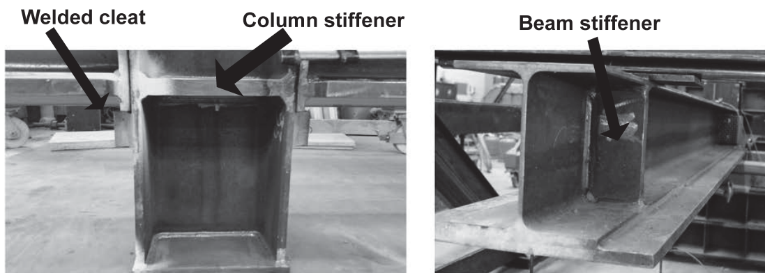
Figure 3.5: Stiffeners in the specimen and welded cleat
