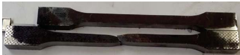
Figure 3.27: Tensile test coupons of endplate
