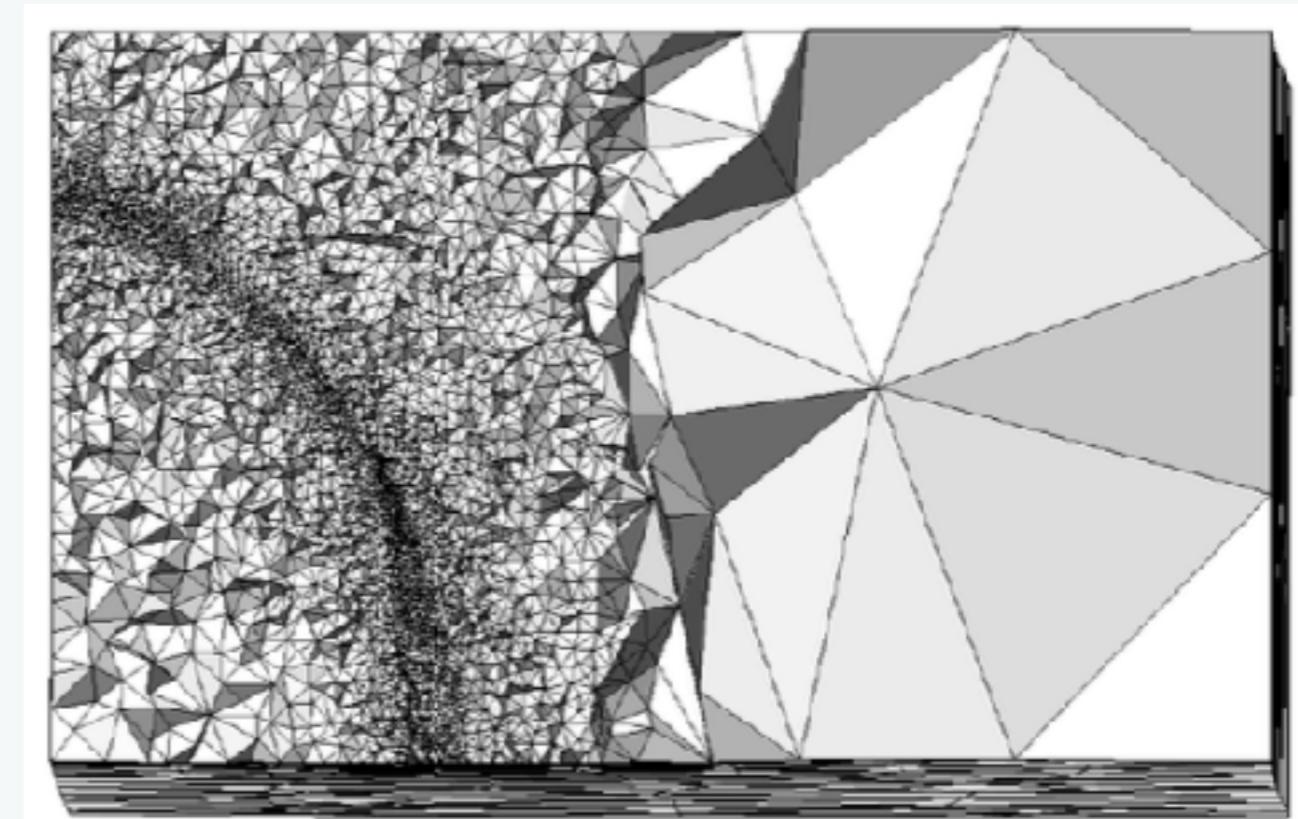
After: determine mesh refinement adaptively using a (goal-oriented) error estimate
