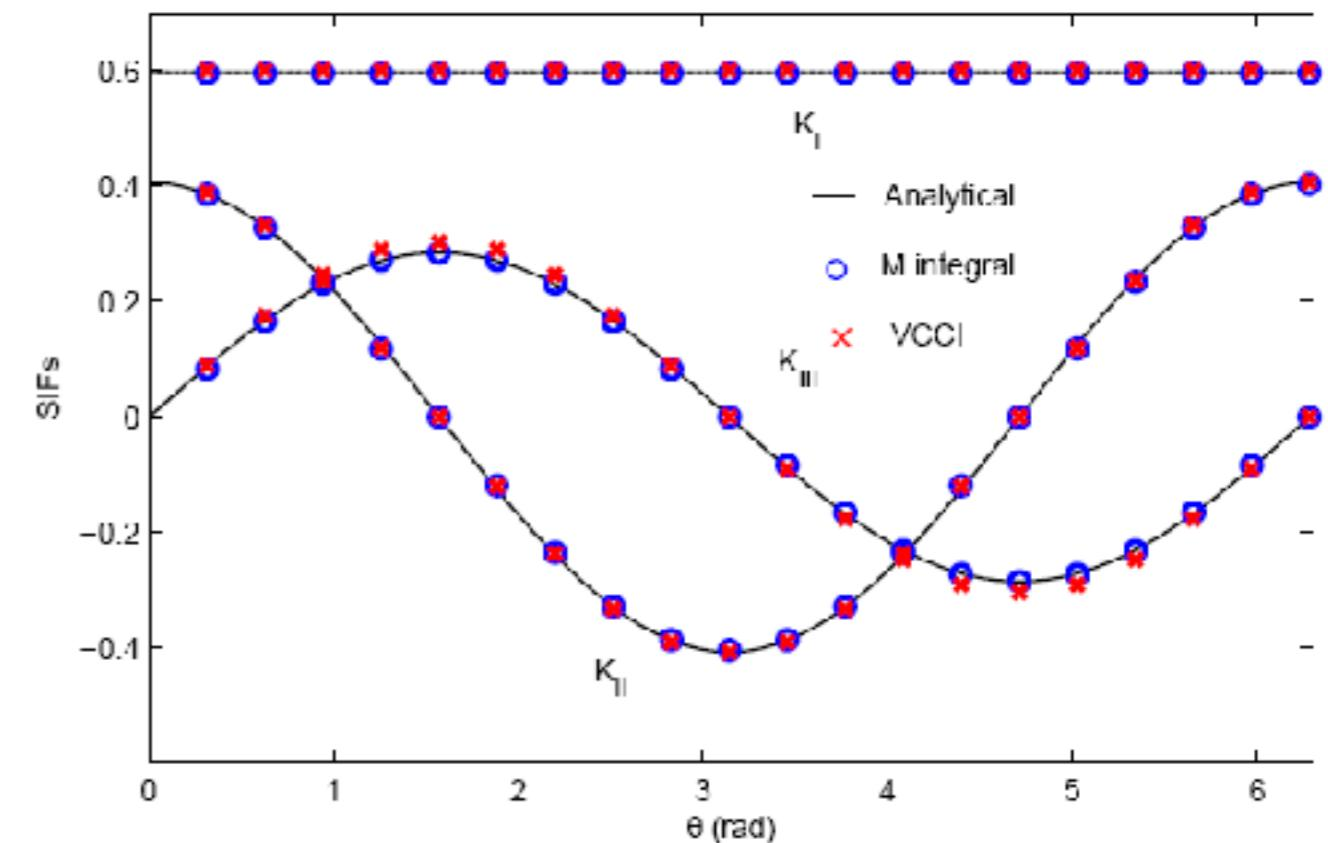
stress intensity factors for penny crack
