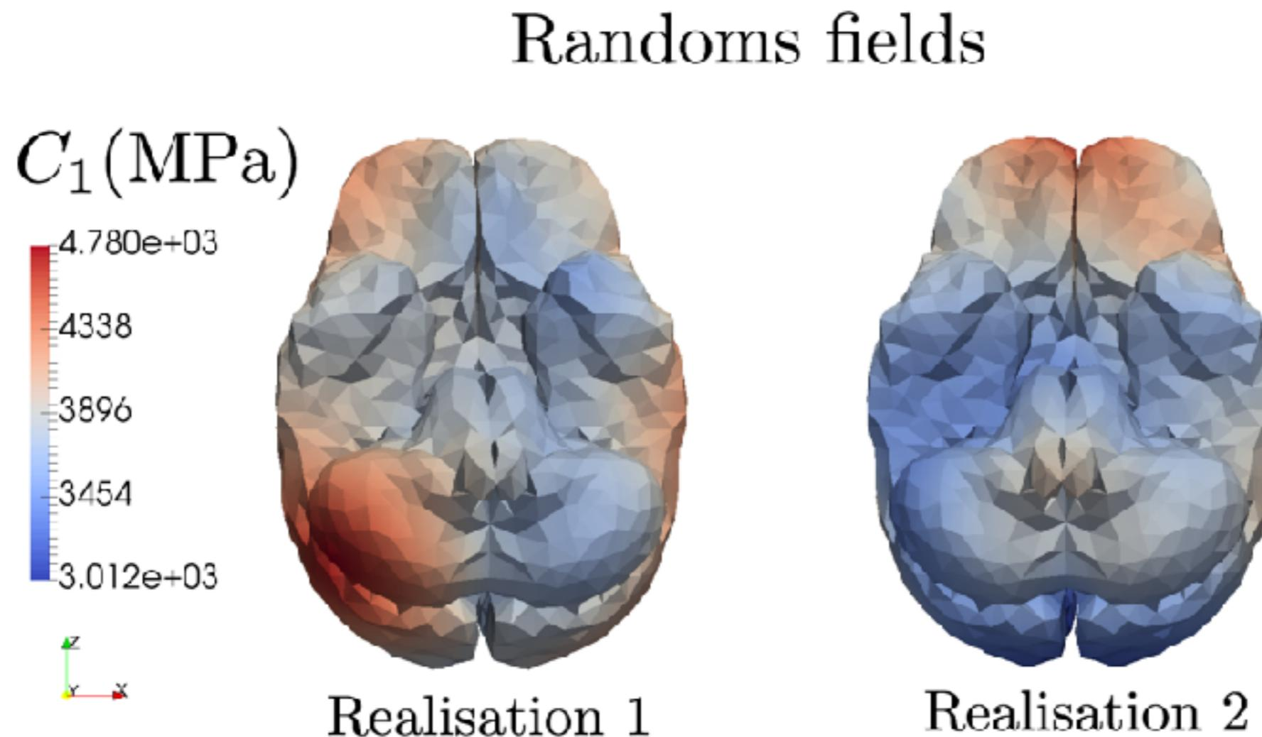
Two realisations of RF, with a log-normal distribution, for the parameter  $C_1$  (in MPa).
