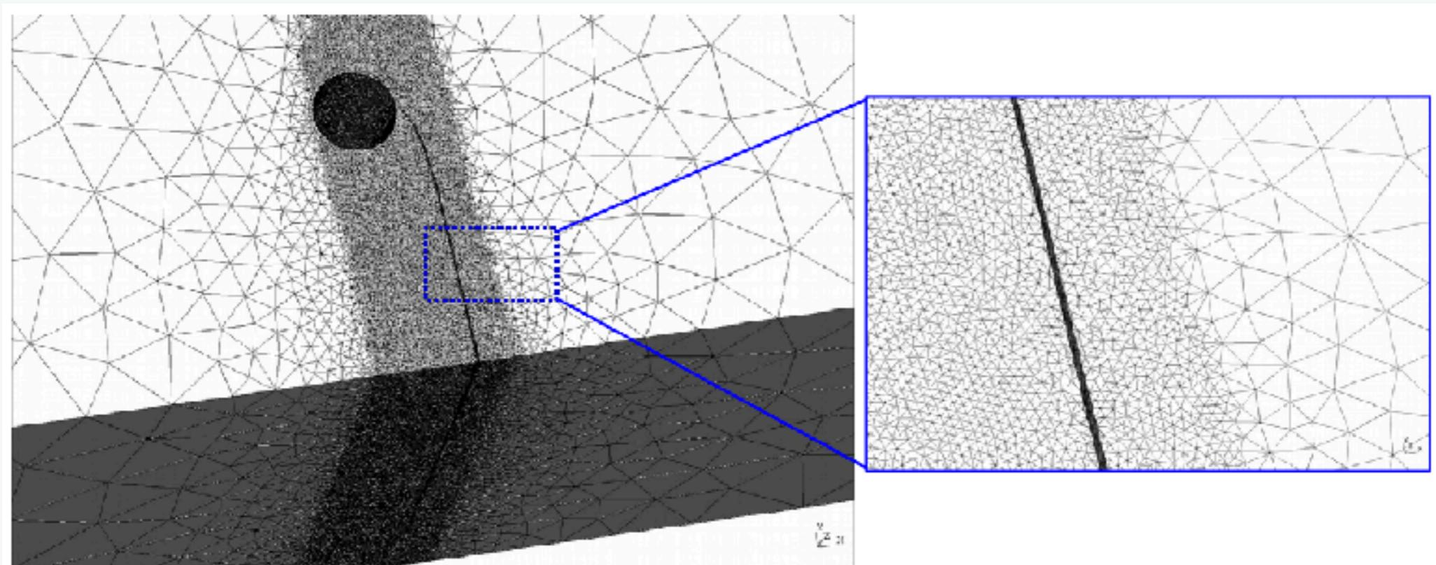
Before: mesh “finely” in the region where the crack is “expected” to propagate
