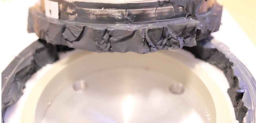
Figure 4.46: Detailed view on the failure pattern of a circular shear test specimen
