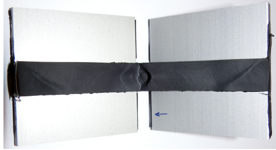
Figure 4.53: Cohesive failure of a H-specimen in tension (specimen ETAG-T-UA-03)
