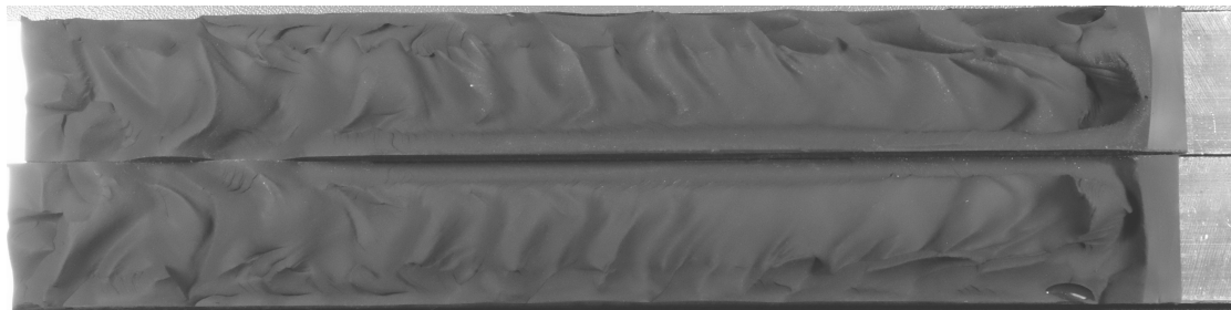
Figure 4.65: Typical failure pattern of a DCB specimen. The pre-crack corresponds to the smooth surface at the right-hand side of the photo.
