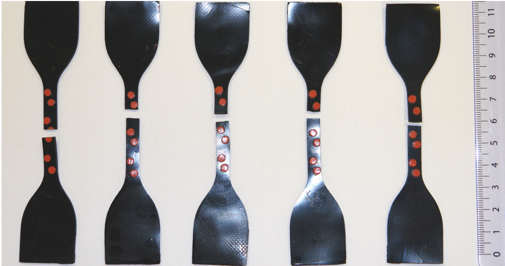
Figure 4.5: Failure pattern of the uniaxial tensile test specimens
