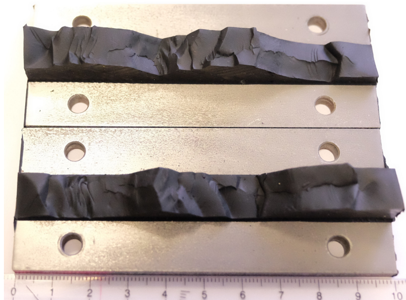
Figure 4.27: Typical failure pattern of a simple shear specimen
