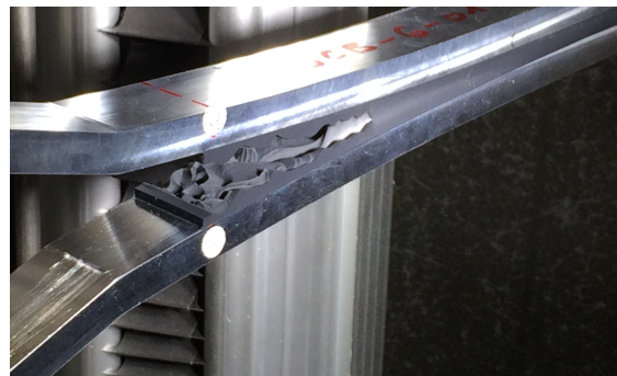
(c) Failure pattern of a DCB-6 specimen
