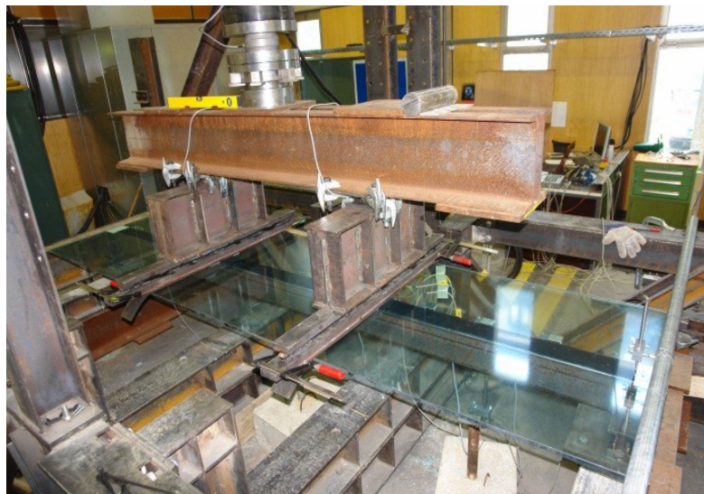
Figure 3.10: Steel to glass composite beam, developed and tested at the University of Luxembourg, picture from Dias (2013)
