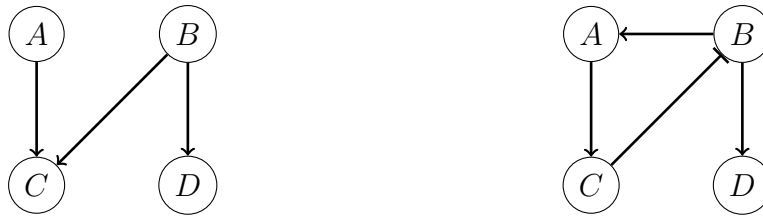
Figure 1.2: Left: An example of a Bayesian network consisting of four nodes. The parents of node C are A and B ; C is independent of D . Thus, P\{C|A, B, D\} = P\{C|A, B\} . Right: An example of a Boolean network consisting of four nodes. An arrow “ \rightarrow ” represents activation while an arrow with a bar ending (“ \dashv ”) represents inhibition. Boolean functions are not shown in this figure. This network structure contains a loop ( A \rightarrow C \rightarrow B \rightarrow A ) while the Bayesian network on the left does not contain any loop.
