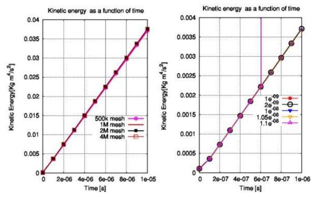
*Figure 4* Dependency of the Kinetic energy from the grid and time step resolution.
