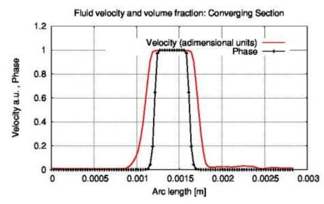
*Figure 6 Fluid solution: velocity and volume fraction profiles along the converging nozzle section.*
