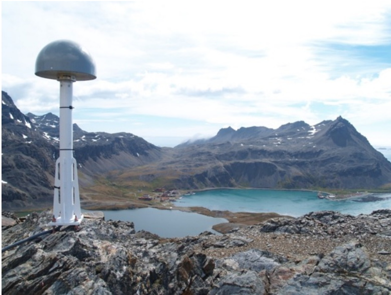
GNSS antenna and mast...good sky view on top of Brown Mt.
