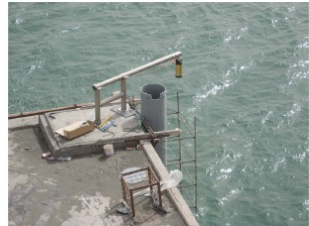
View of the radar sensor arm (viewed from the top of the observatory)
