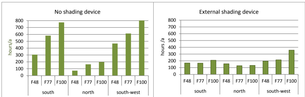
Figure 42: Hours of overheating/a in the office zone produced by a more detailed simulation model
