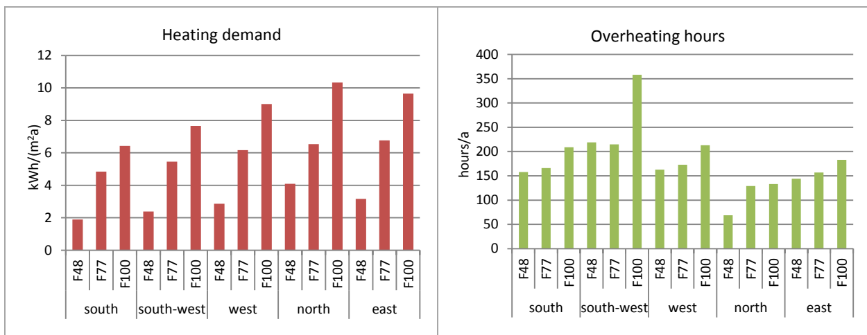
Figure 43: Office zone heating demand and overheating hours with different orientations 19
