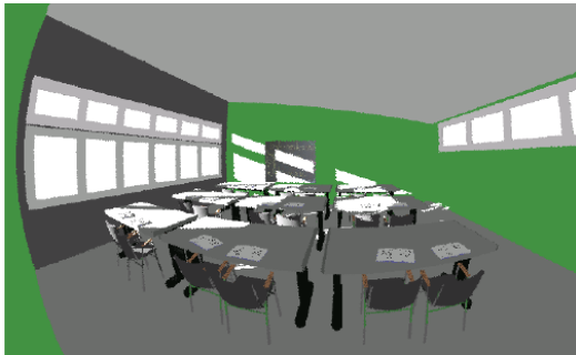
Figure 24: Direct distribution of radiation within a zone [Transsolar-1]
