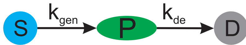
Figure 2.2: A product ( P ) with reactions of generation and degradation. Each reaction has its own rate constant. In principle, a product can have no reactions of generation and degradation. In this case it is assumed that a product concentration remains the same during all time of simulation.
