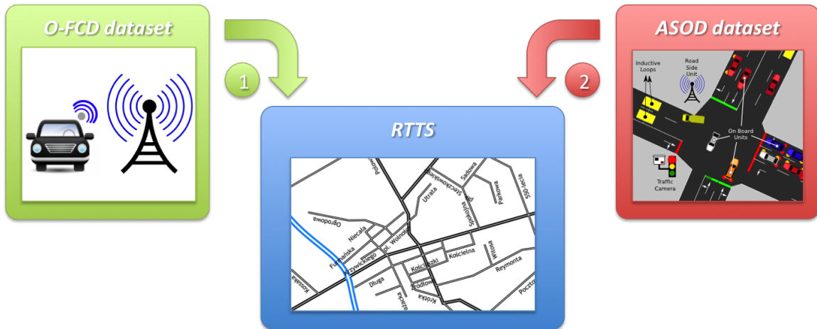
Figure 4.10: RTTS information sources. The two possible datasets are composed of O-FCD and ASOD, FCD included.
