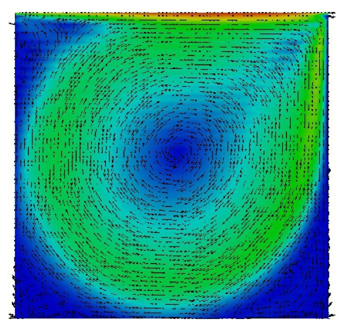
Lid-driven cavity velocity magnitude fields with vectors fields for Reynolds number  $Rey = 10^4$ .
