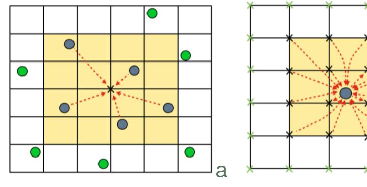
(a) Particle-to-mesh interpolation and (b) mesh-to particle interpolation in 2*D* using an interpolation function with support region 2*h* (shaded in yellow). Blue particles and mesh nodes are within the support region of the centre node/particle and hence assigned onto it. Green particles and nodes which lie outside the support are not considered.
