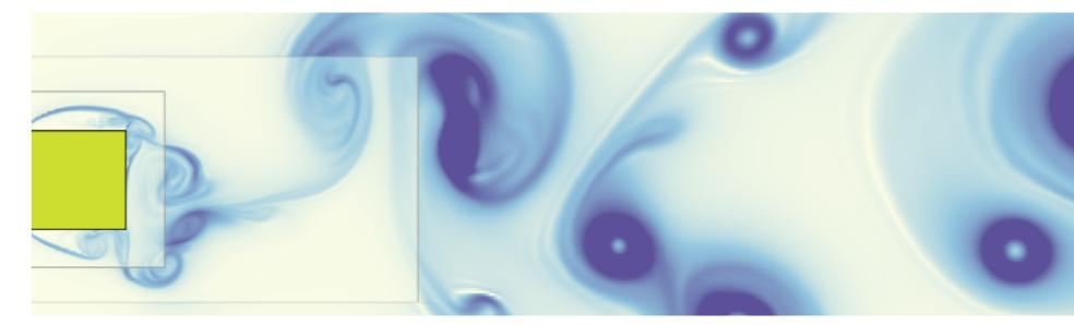
Transported eddy viscosity of an LES simulation of the flow around a square cylinder using the kinetic turbulent energy transport equation
