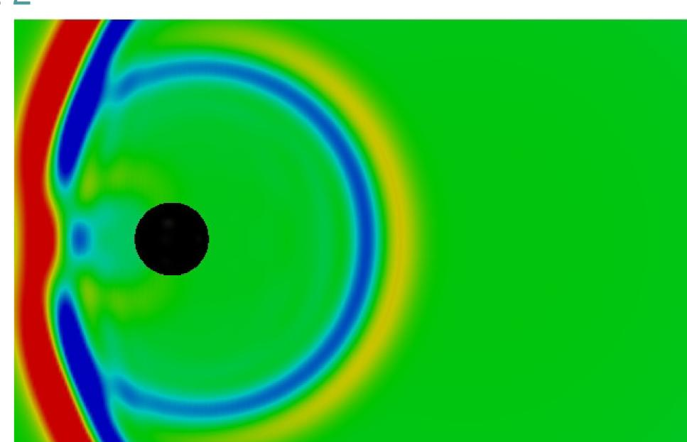
Compressible shock wave perturbation pressure simulation, here we can see the first reflected wave off the solid obstacle.
