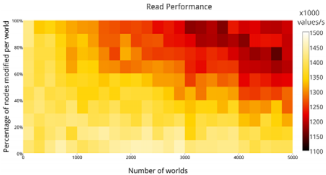
Figure 5.10: Read performance before the divergent timepoint, over several worlds and several percent of nodes modified
