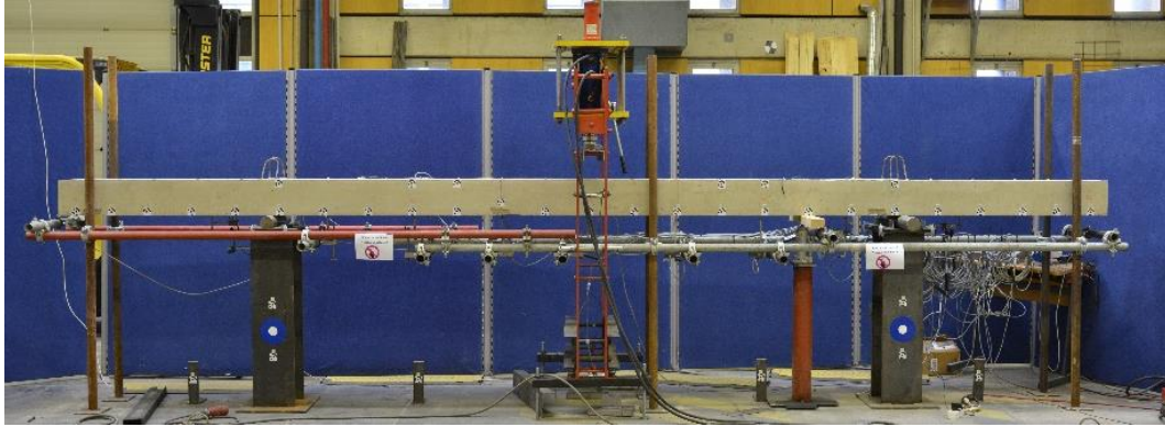
Fig. 1. Laboratory test setup of a reinforced concrete beam
