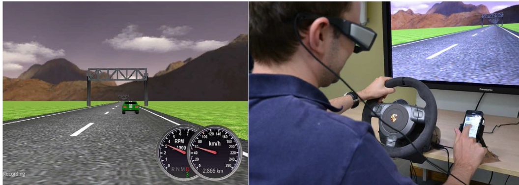
Fig. 1. Experimental task (left) and set-up (right): In half of the trials participants were to follow the lead car while they interacted with a docked smartphone in the driving simulator.
