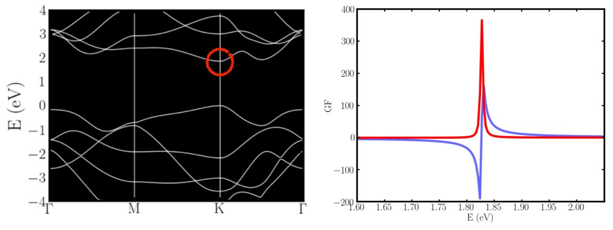
Without lattice-interaction: Electronic states have infinite lifetimes Reality: Lattice-interaction gives them a finite lifetime
