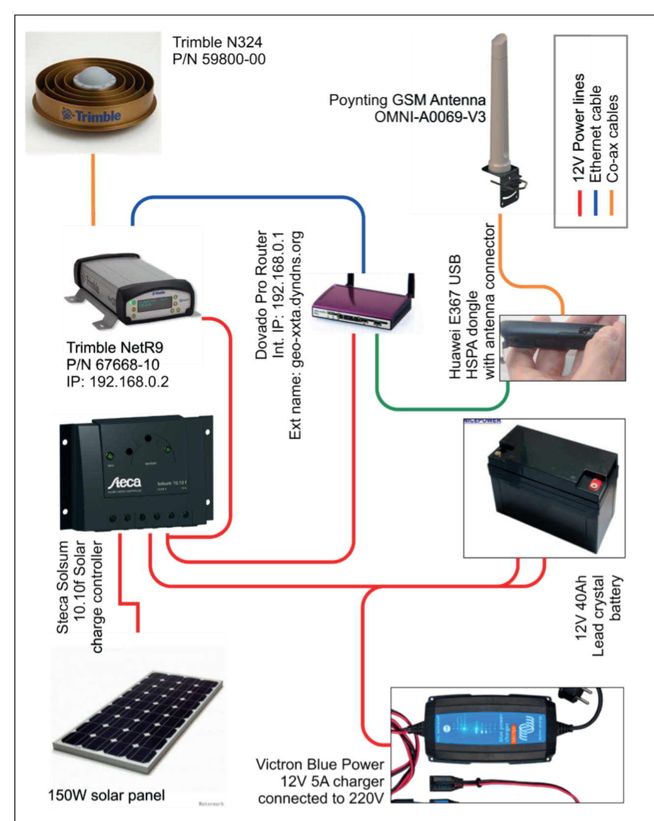
Figure 3: Generic continuous GNSS station layout and diagram.
