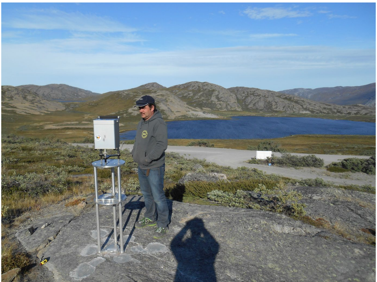
Figure 1. Vertical gravity gradient measurements with a Scintrex CG5 at outdoor absolute gravity station in Kellyville.
