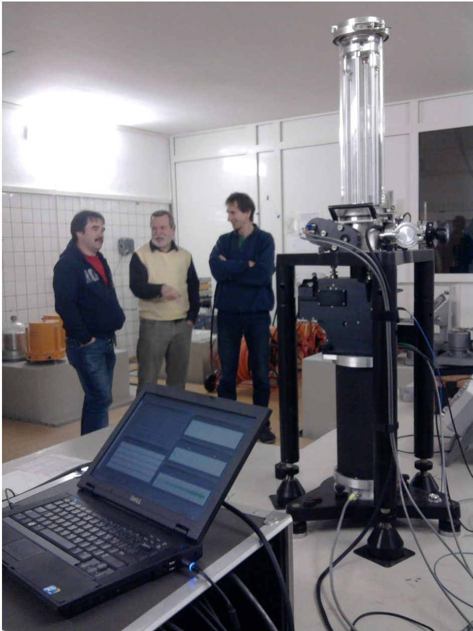
Figure 1. The absolute gravimeter FG5X#216 on the pier AGM, at the Geodynamic Observatory in Moxa.
