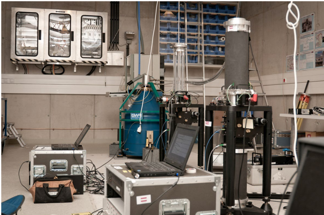
Figure 1. Picture showing from the front to the back the absolute gravimeters FG5-242 and FG5X-216 and the superconducting gravimeter CT-025 on the same pillar.
