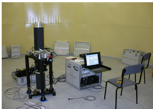
Figure 1. The absolute gravimeter FG5#216 from the ECGS at the Lomonosov gravimetric site.
