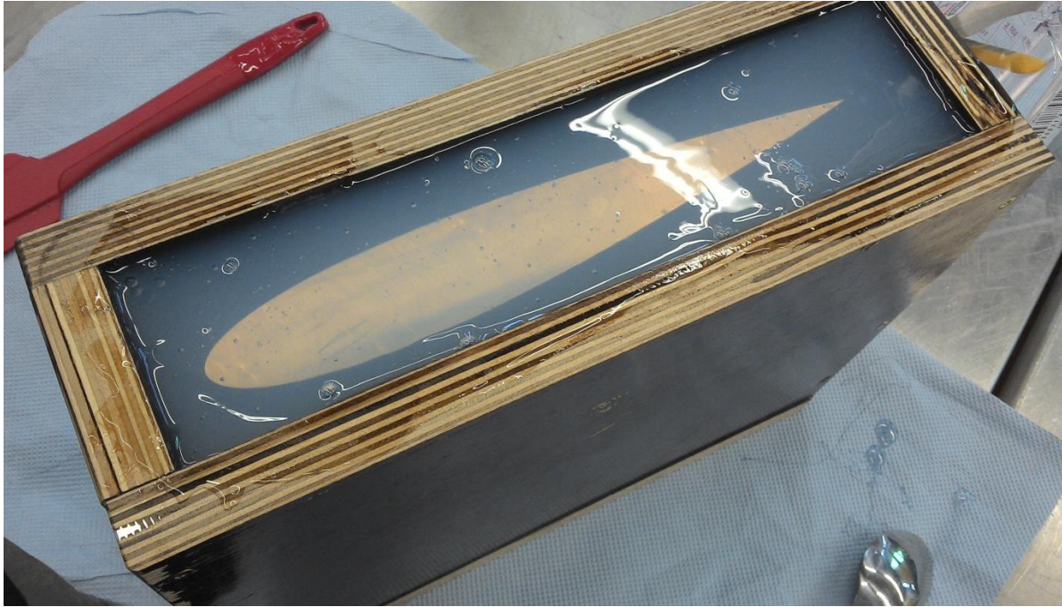
Figure 7. Box filled by silicone to produce the negative silicone form for moulding the PUR foils.
