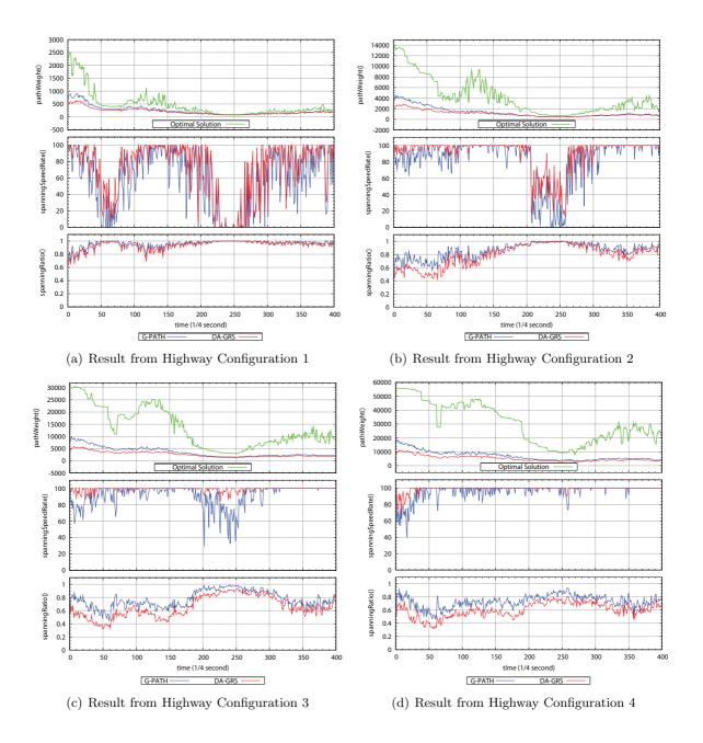
**Figure 5.18:** Result of G-PATH utilizing battery percentage level compare to DA-GRS and optimal value of nodeWeight() function: Highway Mobility Model
