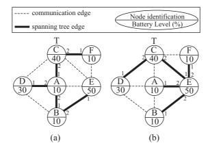
Figure 4.14: An example scenario for Illustrating the details of robustness metrics for percentage of battery level case
