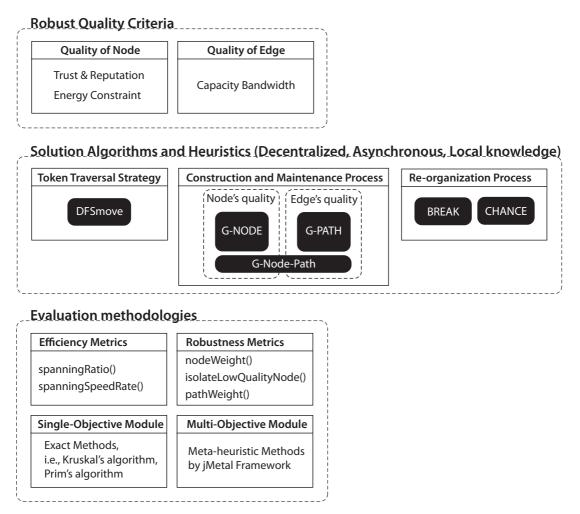
Figure 4.23: Proposed Framework for Topology Management in DT-MANETs based on Spanning Forest
