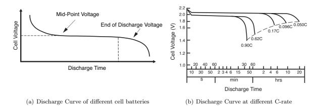
Figure 4.8: General Discharge Curve Characteristic
