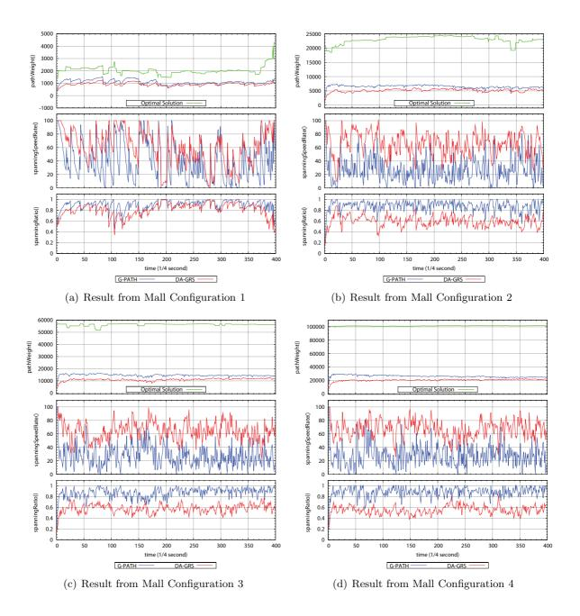
**Figure 5.19:** Result of G-PATH utilizing battery percentage level compare to DA-GRS and optimal value of nodeWeight() function: Mall Mobility Model
