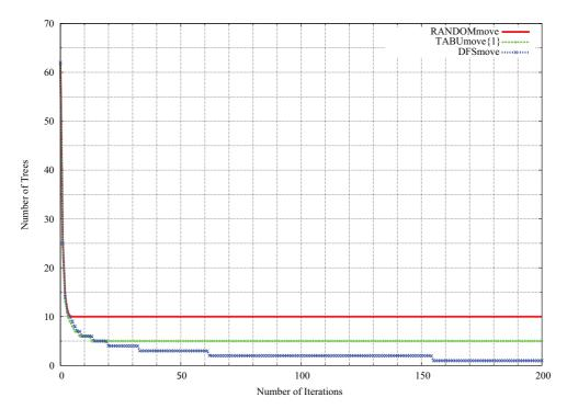
**Figure 5.10:** The result based on 600 runs comparing the number of iteration used in obtaining trees using different strategies (RANDOMmove, TABUmove and DFSmove)
