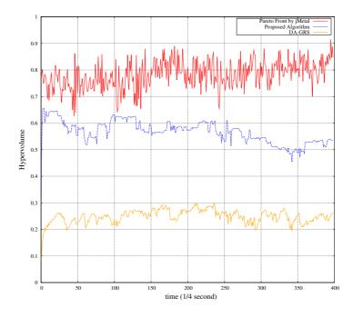
Figure A.36: Hypervolume: G-Node-Path, DA-GRS and Pareto front on shopping mall Configuration 2
