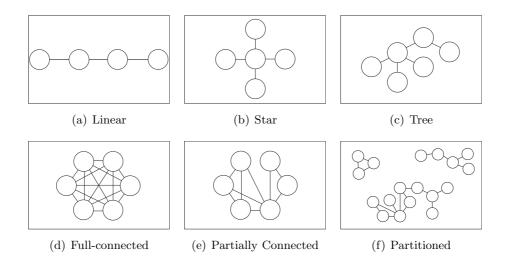
Figure 3.1: Examples of Topology in MANETs
