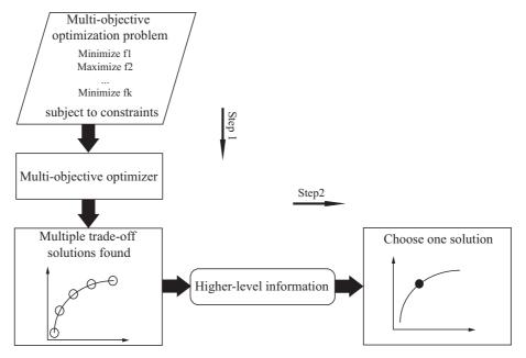
Figure 2.6: Multi-objective optimization procedure
