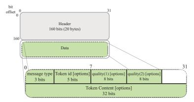
Figure 5.7: Packet Structure used for G-NODE and G-PATH heuristics
