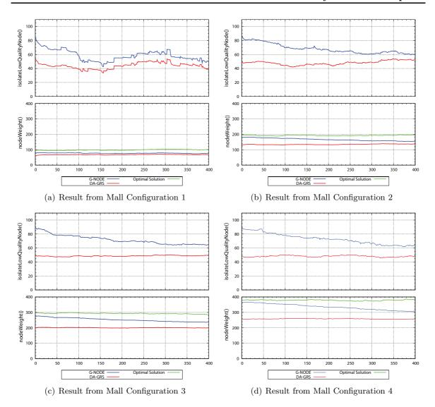
Figure 5.15: Result of G-NODE utilizing trust value compare to DA-GRS and optimal value of nodeWeight() function: Mall Mobility Model
