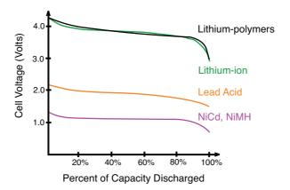
Figure 4.9: discharge characteristic of different cell chemistry [2],[3]
