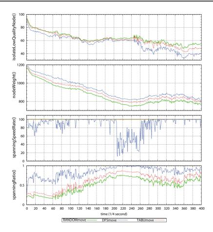
**Figure 5.12:** Comparison of spanningRatio(), spanningSpeedRate(), nodeWeight() and isolatingLowQualityNode() measuring among all studied algorithms in Highway Mobility Model
