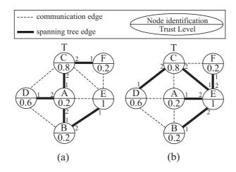
**Figure 4.11:** An example scenario for Illustrating the details of *nodeWeight()* and *iso-lateLowQualityNode()* cost functions
