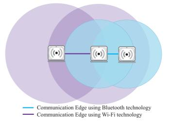
Figure 2.3: Example of three fixed stations equipped with multiple wireless communicating interfaces forming ad hoc networks using different enabling technologies; Wi-Fi and Bluetooth
