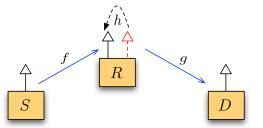
Fig. 1. The system model  $S \to R \to D$ ; the relay node employs a HU architecture (the second antenna at the relay node is used for the FD case).
