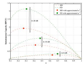
Fig. 5. Instantaneous capacity versus  $\omega$ ; f = 2.83, g = 0.5122, h = 0.91,  $\delta = \{0, 10, 20\}$  dB,  $P_0 = 40$  dB and  $\omega_0 = 0.1$ .
