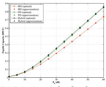
Fig. 6. Ergodic capacity versus  $P_0$ ;  $\sigma_{S,R}^2 = \sigma_{R,D}^2 = \sigma_{R,R}^2 = 1$  and  $\delta = P_0$  dB.
