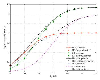
Fig. 3. Ergodic capacity versus  $P_0$  for optimal and approximated time split;  $\omega_{\text{HD}}^* = 1/3$  and  $\omega_{\text{FD}}^* = 1/2$  for constant time split,  $\sigma_{S,R}^2 = \sigma_{R,D}^2 = \sigma_{R,R}^2 = 1$ ,  $\omega_0 = 0.1$ ,  $\delta = 20$  dB.
