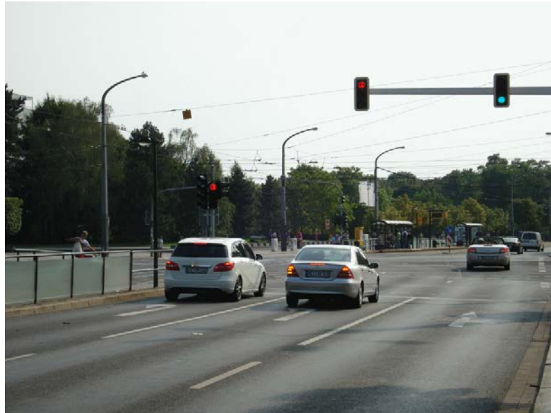
Figure 29: Example of a Protected Left-Turn Regulation with Separate Green Phases for Turning Left Versus Going Straight
