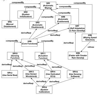
Figure 11 SysML Model for the Rain Sensing Wiper System [14] In the SysML specification [20] deriveReqt has an ambiguous definition which is given as a dependency between two requirements in which a client requirement can be derived from the supplier requirement. Therefore, the mapping from deriveReqt to requires seems the most general one and we take it as a default mapping. For deriveRqt and composedBy we consider that if 'A derivedRqt (or
